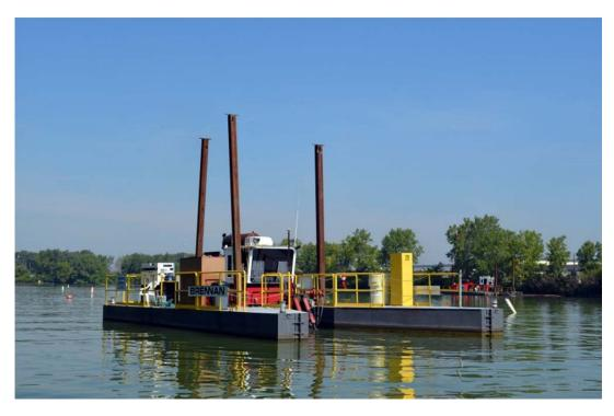
Photo 4. Eight-inch swinging-ladder hydraulic dredge removing non-TSCA sediment.
